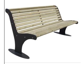
Bench consisting of two sturdy, laser-cut steel side shoulders welded onto elliptical 600x150 shaped bases prepared for fixing the bench to the ground with expansion bolts.
